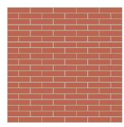
**Stretcher Bond** Using WF format clay pavers (200x48x85mm)
