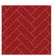
**45° Herringbone** Using DF format clay pavers (200x64x85mm)
