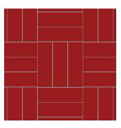
Basket Weave Using DF format clay pavers (200x64x85mm)
