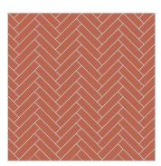
**45° Herringbone** Using WF format clay pavers (200x48x85mm)
