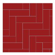
**90° Herringbone** Using DF format clay pavers (200x64x85mm)
