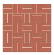
Basket Weave Using WF format clay pavers (200x48x85mm)
