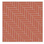
**90° Herringbone** Using WF format clay pavers (200x48x85mm)
