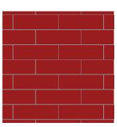
Stretcher Bond Using DF format clay pavers (200x64x85mm)
